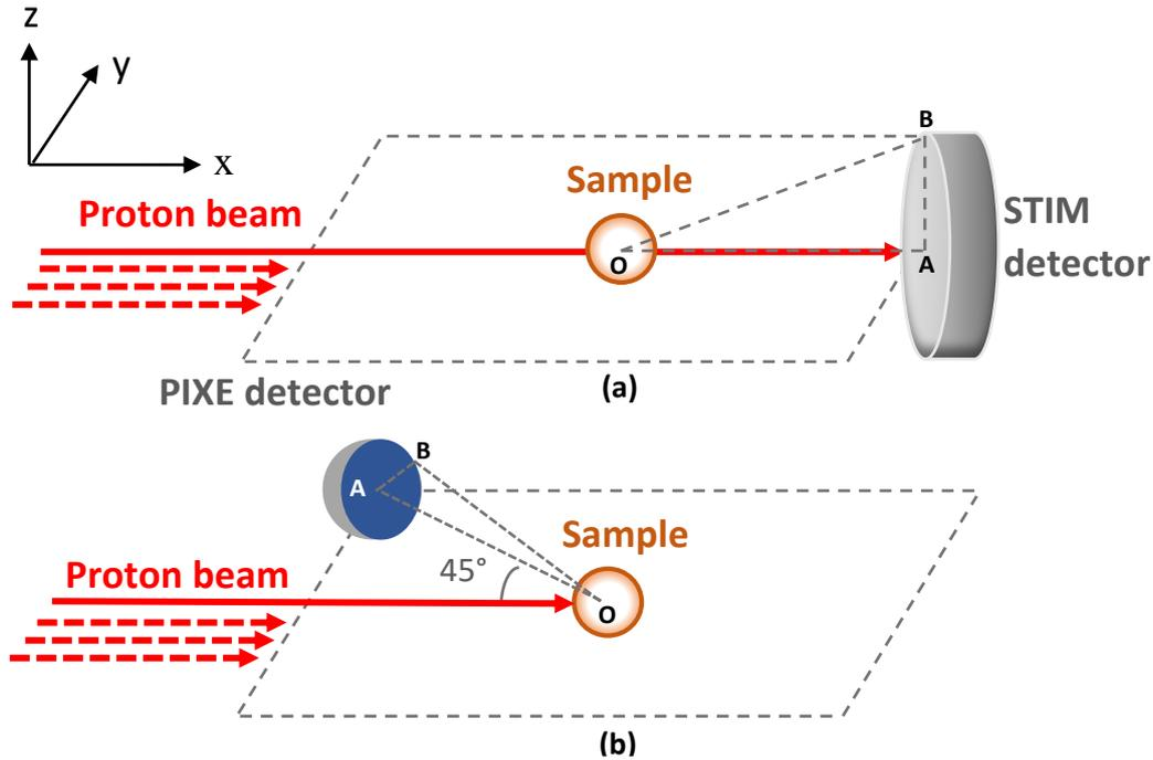
Figure 1. Experimental set-up for STIM-T (a) and PIXE-T (b).
