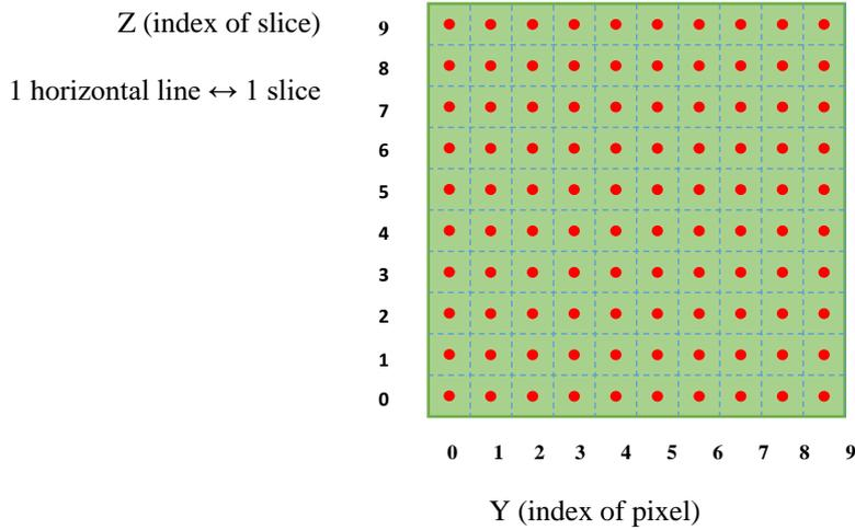
Figure 3. Positions of the beam at a given projection for a scan composed of 10 slices of 10 pixels.
