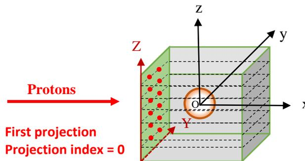
Figure 2. Layout of a simulation of STIM-T or PIXE-T at first projection (projection index = 0).
